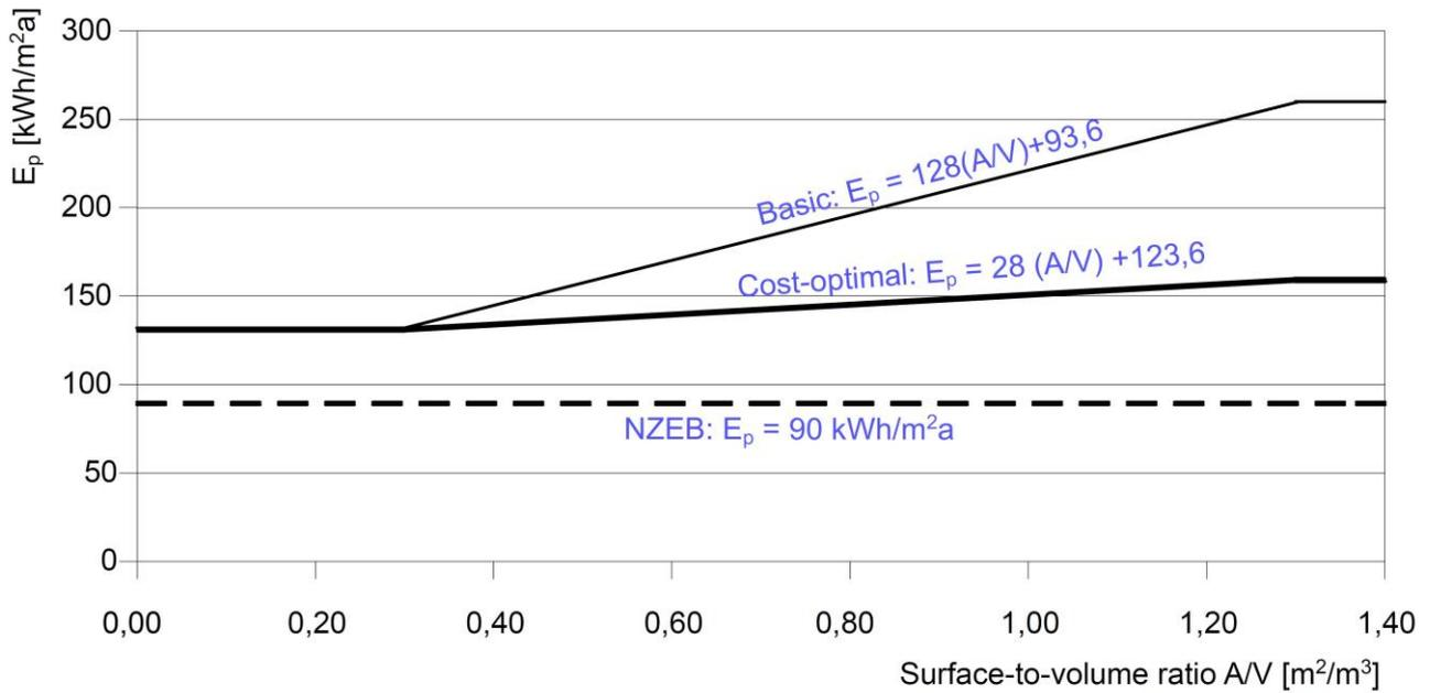
Figure 3. Requirements for the specific yearly primary energy need of office buildings. (Basic: from 2006, Cost optimal: from 2018 (in some cases 2015), NZEB from 2019).
