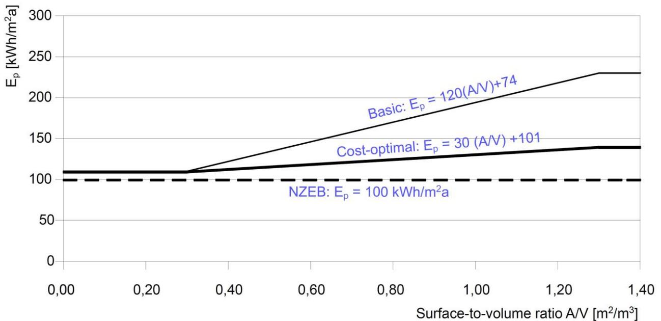
Figure 2. Requirements for the specific yearly primary energy need of residential buildings. (Basic: from 2006, Cost optimal: from 2018 (in some cases 2015), NZEB from 2019.)
