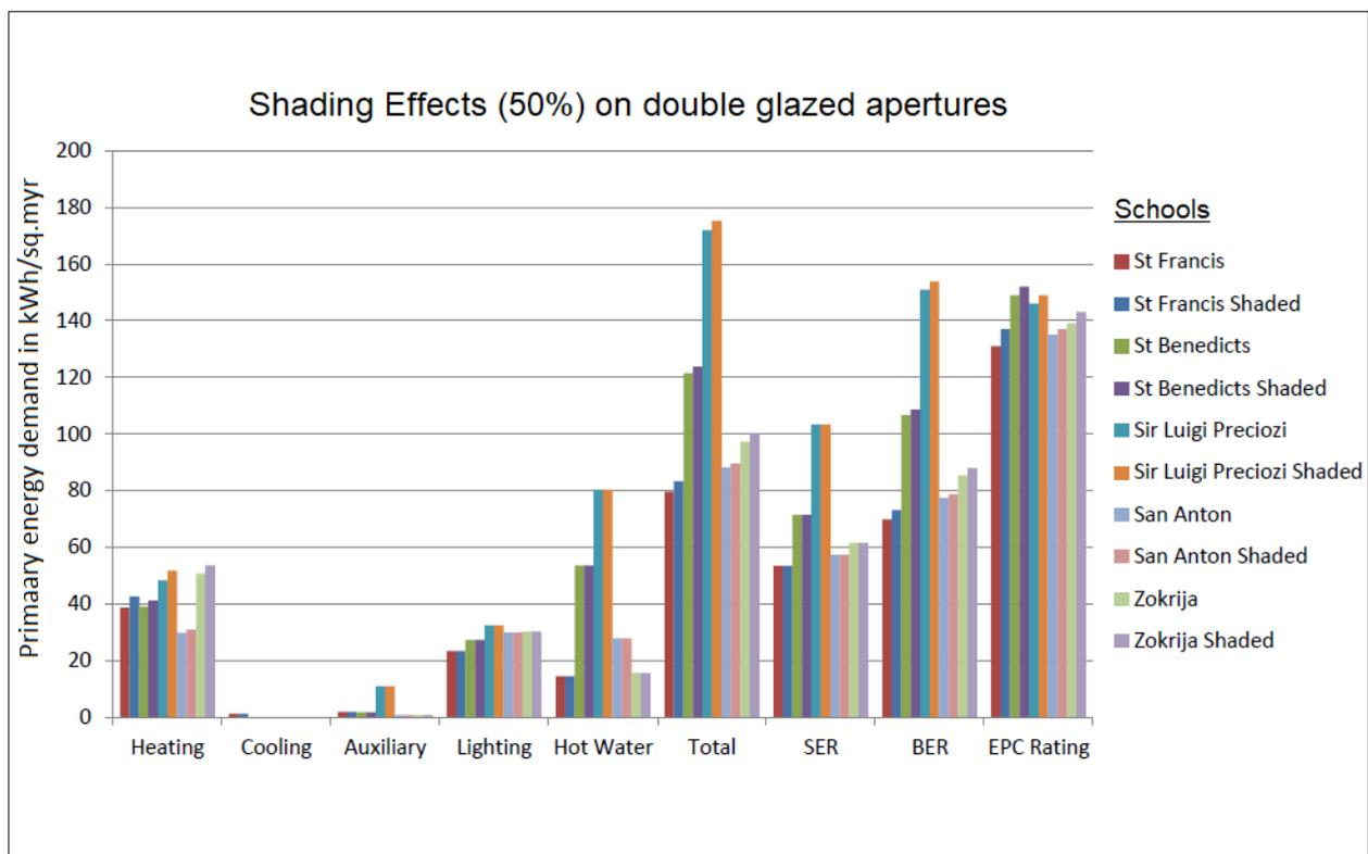
Figure 2. Extract from studies commissioned to enhance minimum requirements, showing results divided by energy use for simulations carried out for shading effects in schools.
